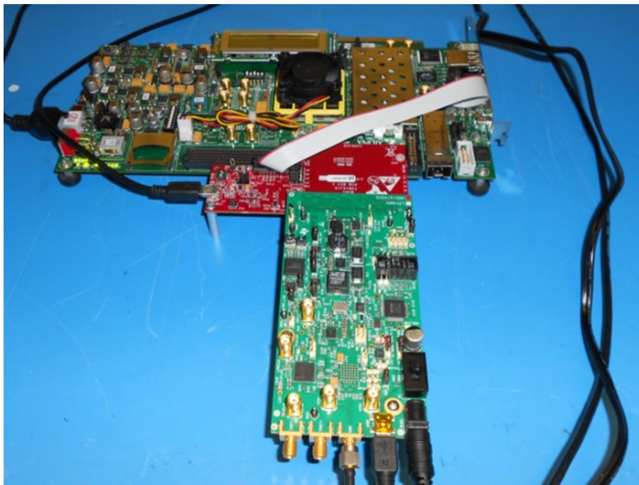
Figure 18. ADC12J4000EVM, TSW14J10EVM and VC707 Board
